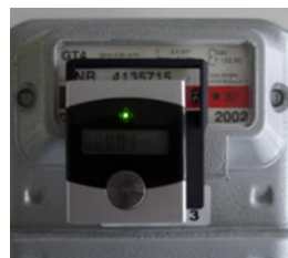
EnergyCam mounted with a Gas Meter Adapter Frame on a gas meter
