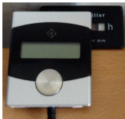
EnergyCam mounted on a Müller time counter
